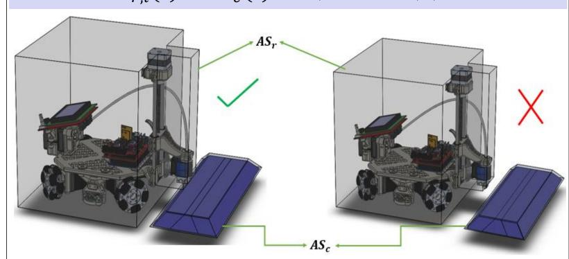
The schedule that results in collision free printing is simulated and the printing can begin.
