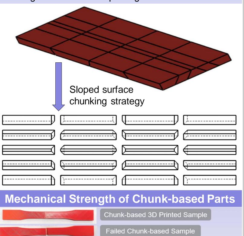
Failed Reference Standard 3D Printed Par
