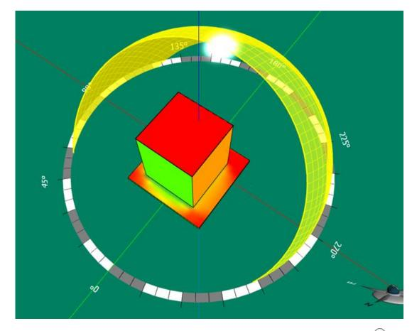
Figure 6. Energy3D's Calculate the Energy of the Day' tool can show the distribution of solar radiation on horizontal and vertical surface areas.
