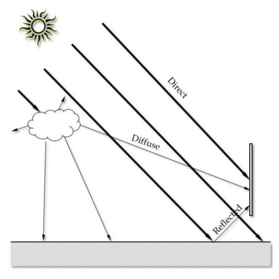
Figure 9. Direct, diffuse, and reflected radiation onto a vertical surface.
