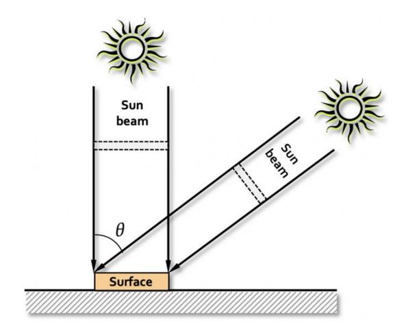
Figure 5. The projection effect on a horizontal surface. The sizes of the dashed areas represent the amounts of solar radiation that the surface receives at the two angles.
