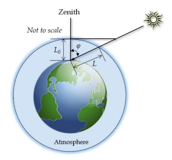
Figure 7. The attenuation of solar radiation in the atmosphere depends on the travel length.
