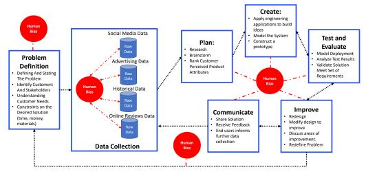
Figure 1: The Potential Bias that can be Introduced in the Engineering Design Process
