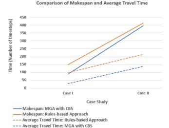
**FIGURE 8:** The changes in makespan and average travel time obtained using different approach for two case studies
