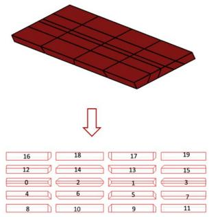
**FIGURE 5:** A rectangular bar with chunk lines shown for visual reference and its exploded view of chunks from top view with marked chunk number
