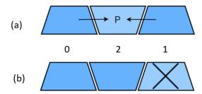
**FIGURE 2:** (a) Rule of geometry indicates that chunk 0 and chunk 1 should be printed before chunk 2 (b) Possible issues resulting from the lack of geometric rule where, chunk 1 cannot be printed if chunk 2 is printed first.
