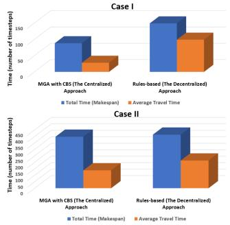
**FIGURE 7:** The makespan and average travel time by robots in both decentralized and centralized approach.
