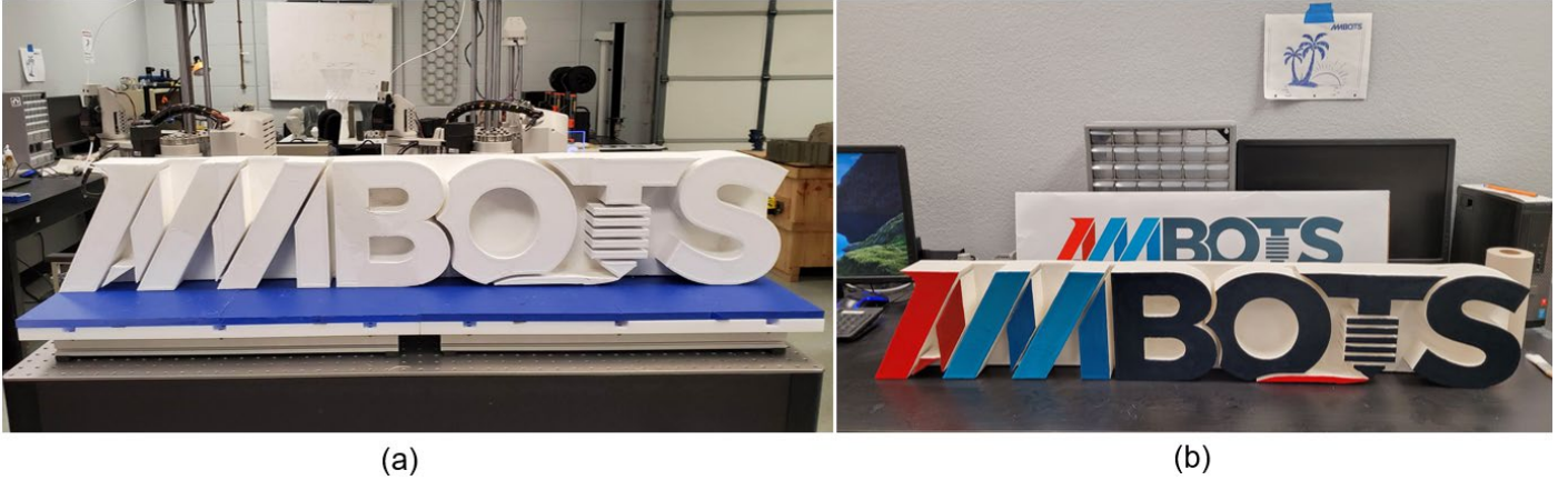
Figure 14. (a) AMBOTS logo printed using two SCARA printers (b) Result after post processing
