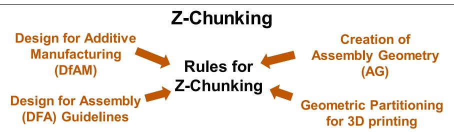
Because robots can not be moved infinitely in the Z direction, as they can in the XY direction, tall objects must be divided into layers, or Z-Chunks, which are printed at different locations are reassembled. For this reason, Z-Chunking is not only a partitioning problem but also an **Assembly** Problem.
