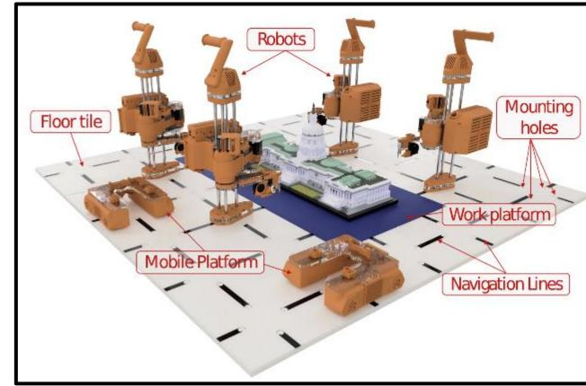
Swarm robots can manufacture arbitrarily large parts, calibrate themselves, and acquire  $\triangleright$ new manufacturing capabilities by switching their end-effectors.
