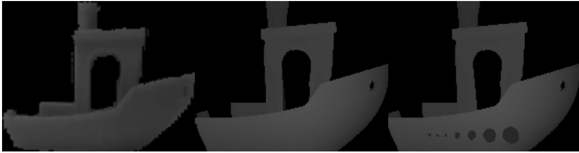
Figure 26: Masks of 3DBenchy. Left: Mask generated from camera image, Middle: Mask generated from correct STL file, Right: Mask generated from altered STL file.
