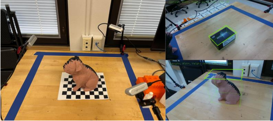
Figure 16: Intel Realsense calibration. Left: Full calibration setup, Top Right: Object detection with a simple box. Bottom Right: Object detection of complex shape.
