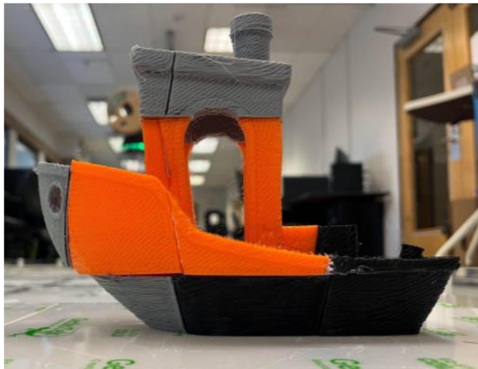
Figure 11: Assembled model of 3DBenchy test case (orange: Printer 1, black: Printer 2, gray: Printer 3).
