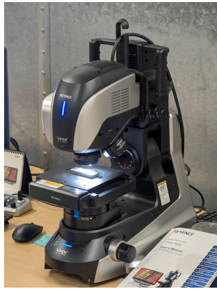
(a) A Keyence VHX 7100 digital microscope.
